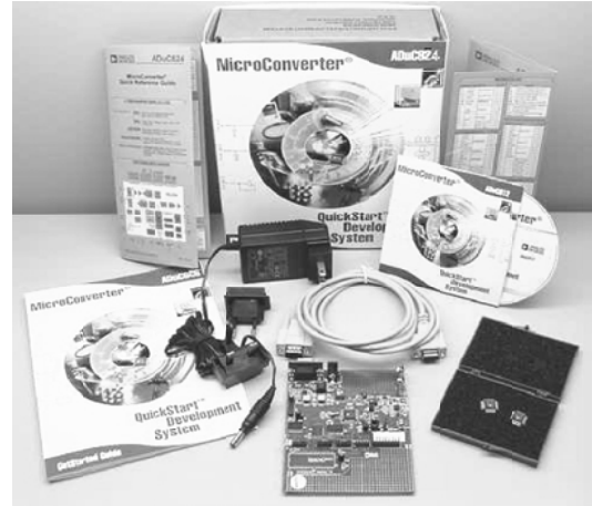
Figure 47. Components of the QuickStart Development System
